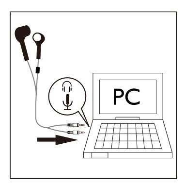
Connect the headphone plug to the  $\bigcap$  socket and the microphone plug to the  $\Psi$  socket of your computer.
